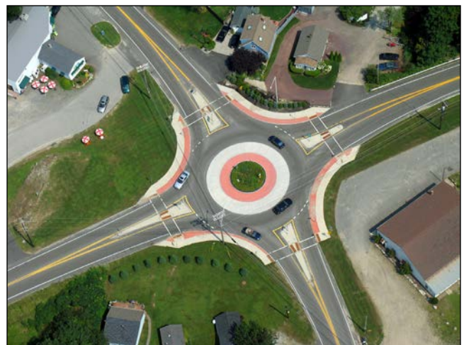
Example of a single lane roundabout in Keene City, New Hampshire. Photo source: New Hampshire Department of Transportation: www.nh.gov/dot/org/projectdevelopment/highwaydesign/roundabouts/index.htm
