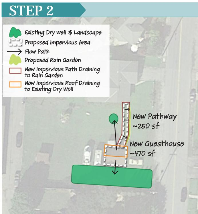
Figure 4-2. Step 2: Prescriptive Design Measure Sizing
