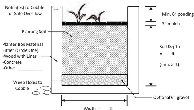
Note: Include weepholes, underdrains, etc as needed to ensure that ponded water completely drains within 4 days.
