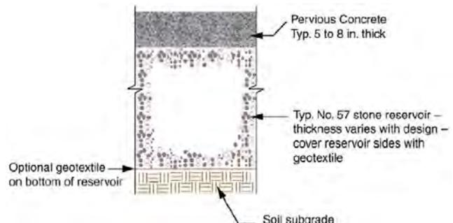
Typical Porous Concrete Pavement Section
