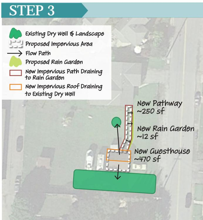
Figure 4-3. Step 3: Prescriptive Design Measure Sizing
