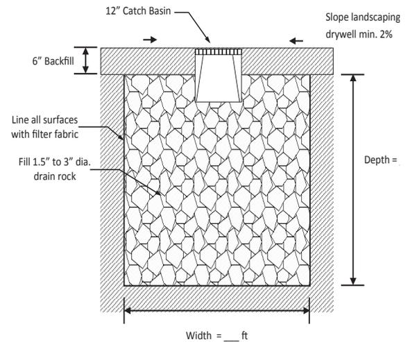
Drywell Section Example Detail for indirect / overland storm-water flow
