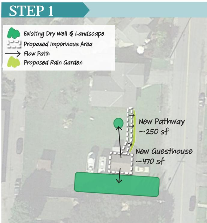
Figure 4-1. Step 1: Prescriptive Design Measure Sizing
