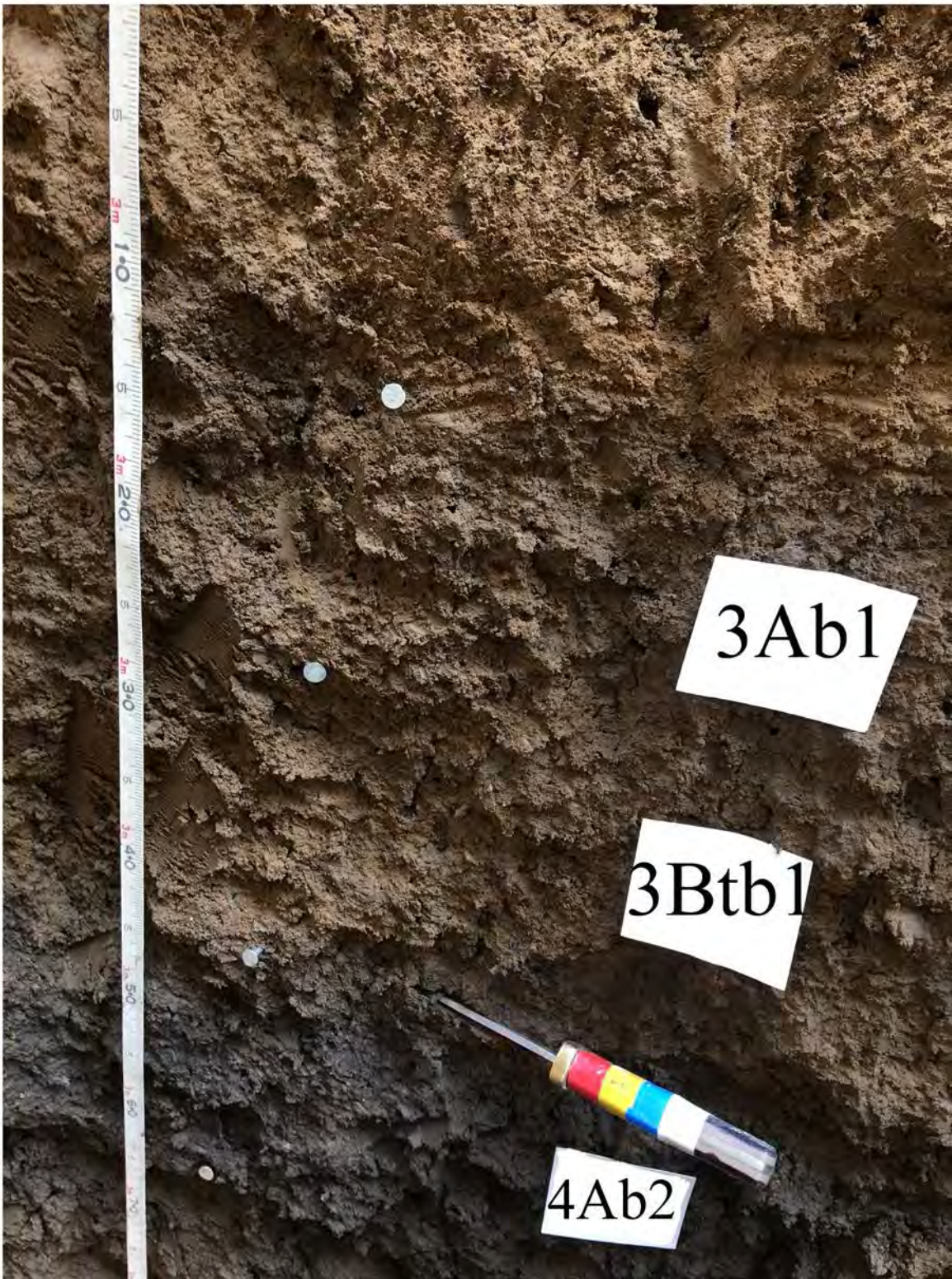
Figure 4. The short-duration b1 and b2 paleosols. The top 1cm of the Ab2 horizon had a C-14 age of 5.3 ka (Table 2). The b2 paleosol was estimated to have a t_d of 1 ka, yielding a t_o age for the profile of 6.3 ka.
