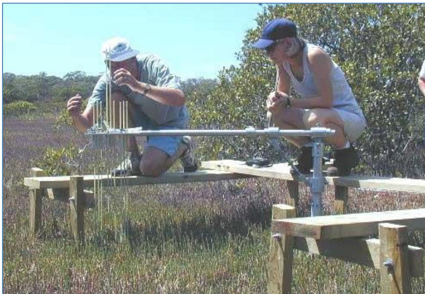
The benefit of using a SET to monitor changes in wetland elevation is that it can provide a highly accurate and precise measurement of wetland elevation. The drawbacks are that the initial set-up and equipment costs are relatively high, and using the equipment is time consuming and requires specialized training. Furthermore, the SET is typically placed in vegetated marsh, rather than mudflats. The marsh plain may not be as sensitive to changes in sediment supply as mudflats.
