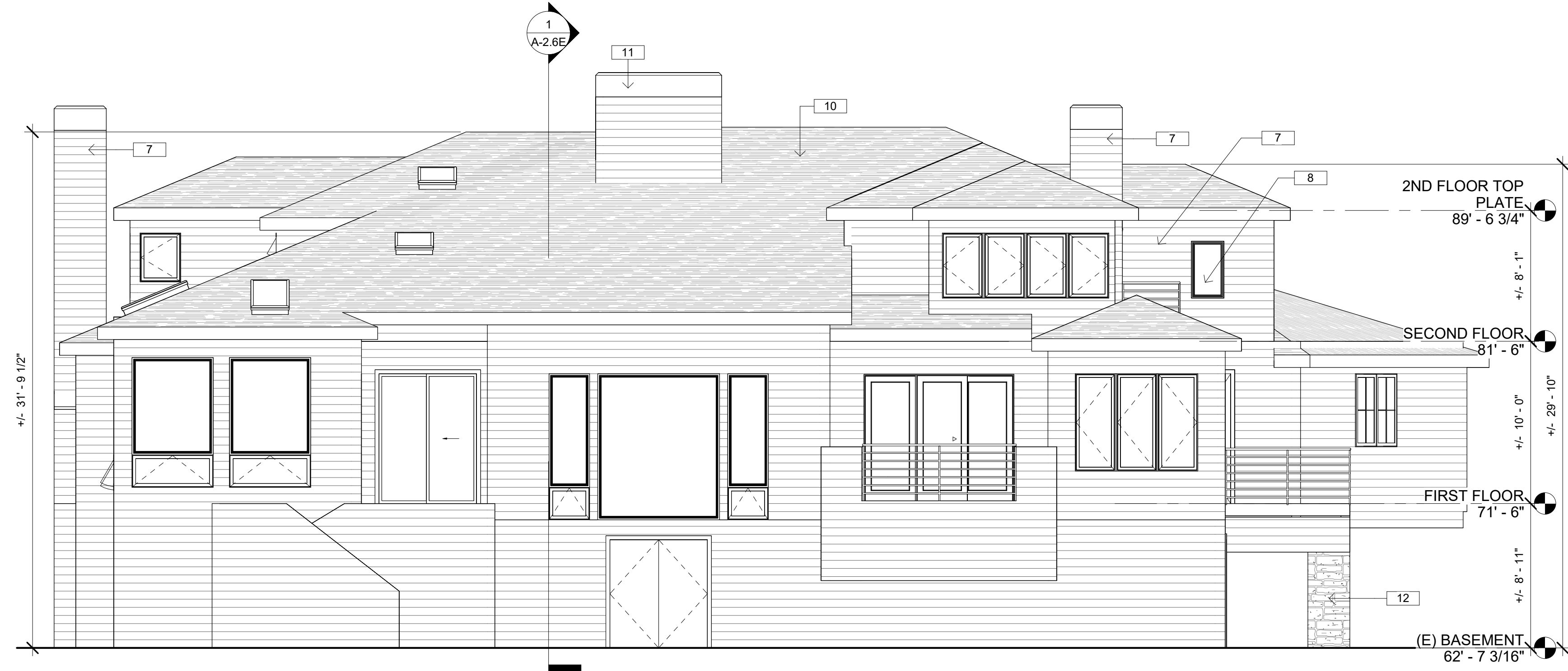
4 (E) NORTH ELEVATION (REAR) 3/16" = 1'-0"
