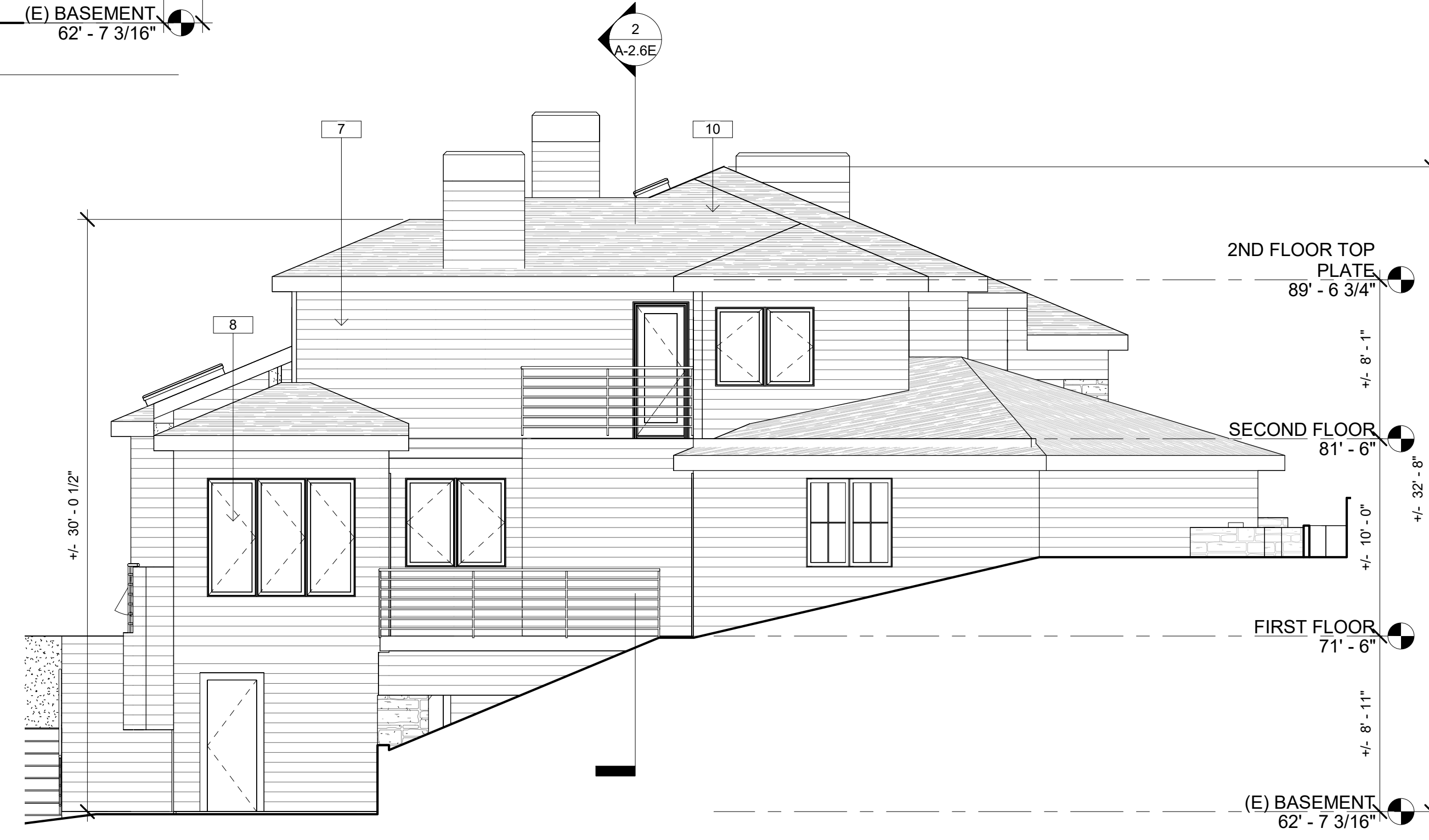
3 (E) WEST ELEVATION (LEFT) 3/16" = 1'-0"
